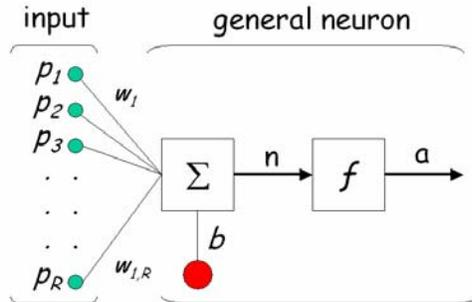
**Figure A-1. The architecture of one layer in a multilayer feedforward perceptron.**
