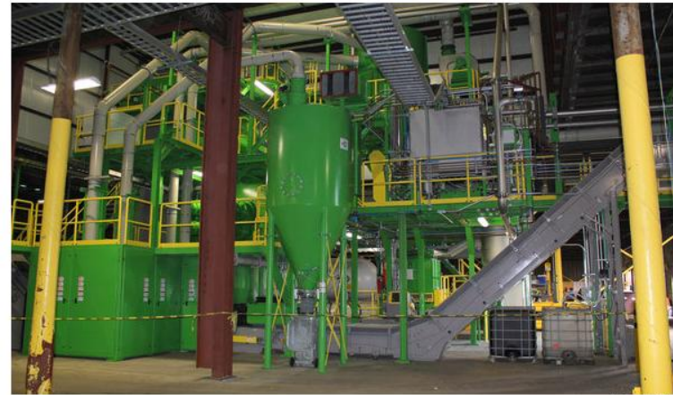
A machine in Philadelphia can dismantle a refrigerator in 60 seconds for recycling, removing 99.8 percent of the coolant.
