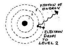
NOTE: Be sure that you depict the **ELECTRON leaping between energy levels**, NOT a photon! The electron emits or absorbs a photon of energy, not the other way around. Also be sure you show the photon being EMITTED if the electron leaps to a LOWER energy level. (Or, if the question asks you to show what happens when a photon is ABSORBED, show that the electron leaps to a higher energy level.)
