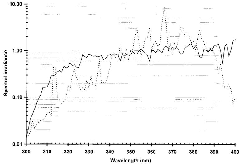
**Fig 1.** Spectral irradiance of the metal halide lamp used in this study (*dotted line*) as measured with a spectroradiometer (model SR3010-PC, Macam Photometrics, Livingston, UK) and compared with a zenithal standard sun spectrum (DIN 67501) (*solid line*).
