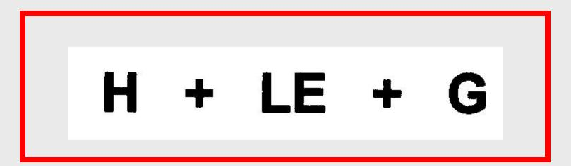
Conduction Convection Phase changes: (latent energy ←→ sensible heat)
